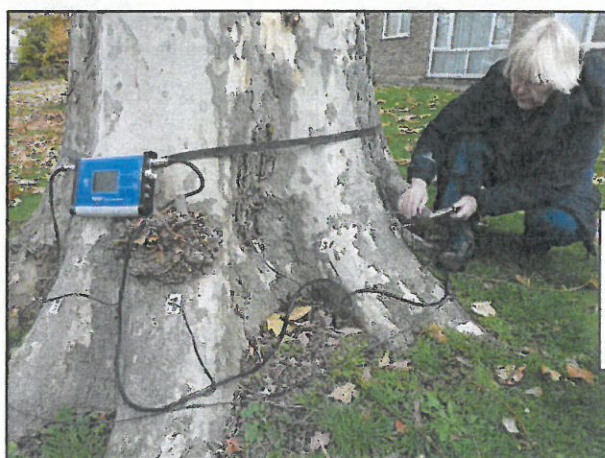
The latest version of the Picus in use at the base of a London plane tree
